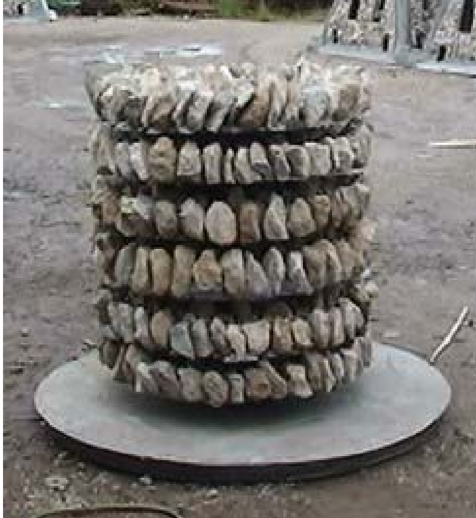
Figure 5. New artificial fish reef constructed by Reefmaker which will be deployed at the Northern Neck and Poquoson reef sites, as well as others to be determined in consultation with VMRC and recreational fishers. Note: The spacing between reef layers will be increased in alternating layers to provide suitable shelter for larger fish.
