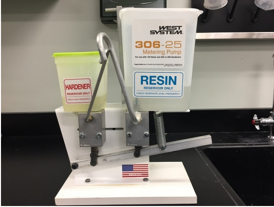
Figure 12: The pump for mixing Epoxy resin and hardener at a ratio of 5:1.
