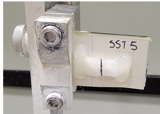
Figure 7: A resin block with a marked otolith is mounted on the chuck but the right end of the block and tag are not clamped together, yet.
