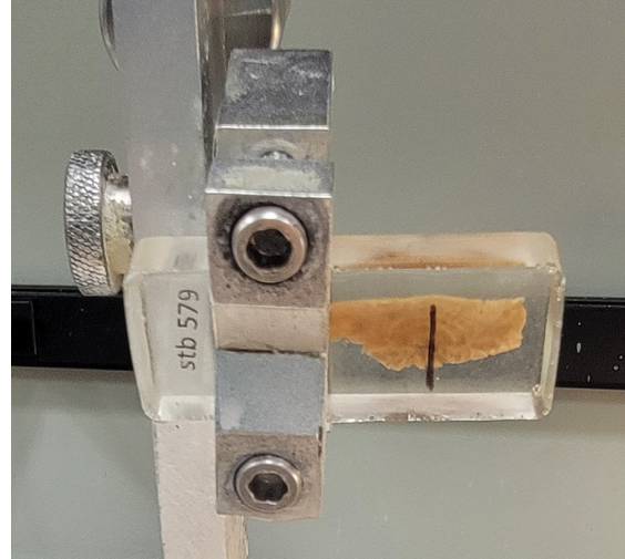
Figure 17: Marked resin with otolith embedded is mounted in the chuck of the saw arm.
