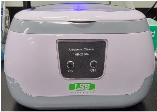
Figure 6: Ultrasonic cleaner is used to clean Striped Bass scales before pressed.
