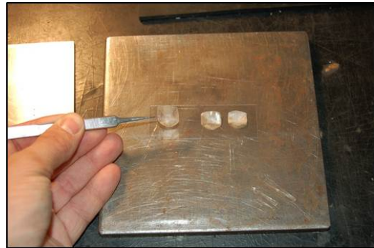
Figure 7: Placement of the acetate slide with scales on the bottom plate, and the rough-side of scales facing down with posterior regions pointing away from the technician.
